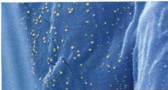
Scanning electron microscope image of silver nanoparticles on the surface of cotton. The silver helps cotton fabric resist microbial growth. Magnification about 12,000x. Story begins on page 14.
